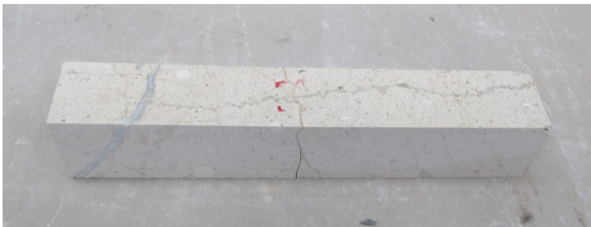
Figure 1. Representation of a specimen after frost resistance and flexural strength test
